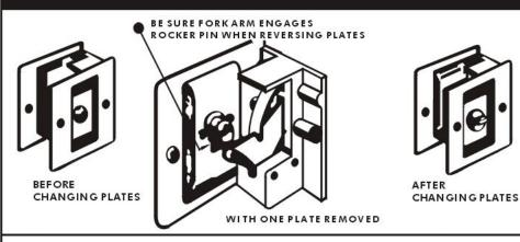
When it is desirable to reverse outside plates on lock assembly, firstremove machine screw on each side-change plates from side to side ( making sure that fork arm engages rocker pin )and re-assemble.
