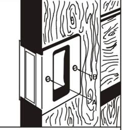
(A)Fasten machine screw which tightens and automatically aligns pull.(B)Insert wood screw and tighten.
