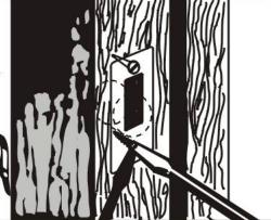
Screw strike plate into position using #6 × 3/4 " Ig. Flat head wood screws.
